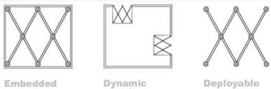
Figure (1) Kinetic structure categories(20)
